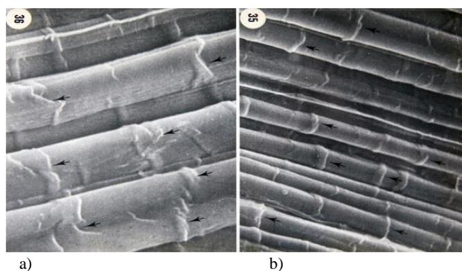
Fig. 2. Archival SEM images from [4] illustrating the systematic presence of nodal markings on individual flax fibres (shown by black arrows) that were obtained at the magnification of a)  $\times 1645$  and b)  $\times 871$ . Typical diameter of the flax fibre lies in the range  $19\ \mu\text{m}$  to  $20\ \mu\text{m}$ .
