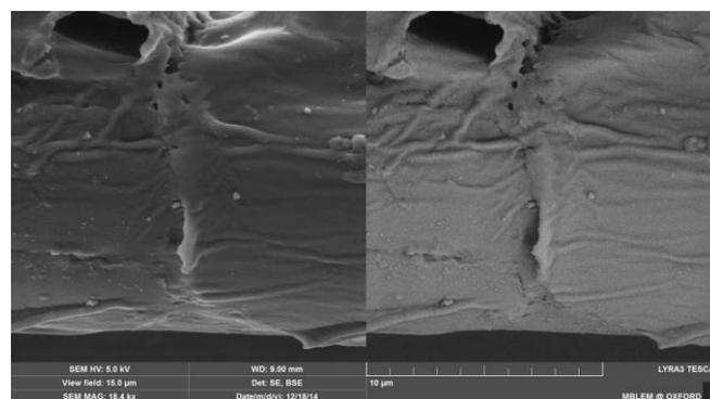
Fig. 4. Higher magnification SEM images of fibre surface in the vicinity of a nodal marking line viewed using SE and BSE detectors.
