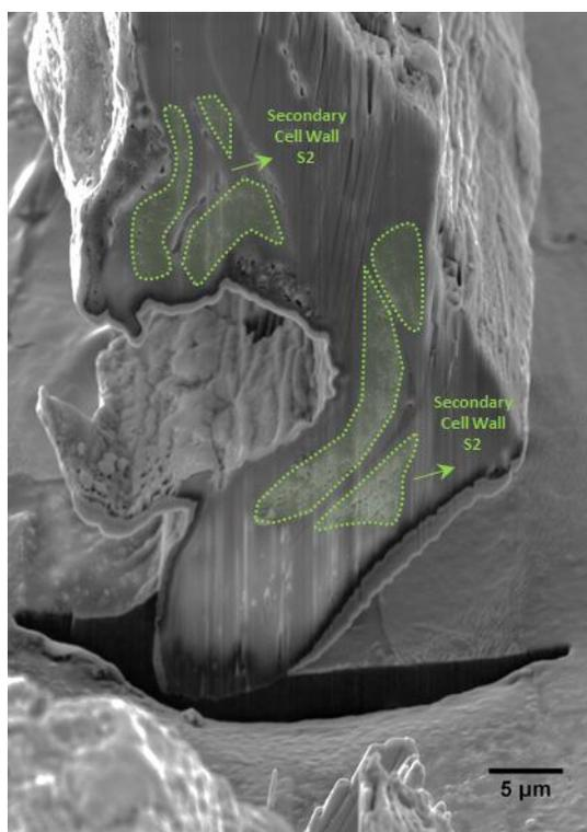
Fig. 7. FIB-SEM cross-sectional image that reveals some details of the secondary cell wall structure (S2) within the etched “islands” identified by the shaded regions surrounded by the green dotted lines.
