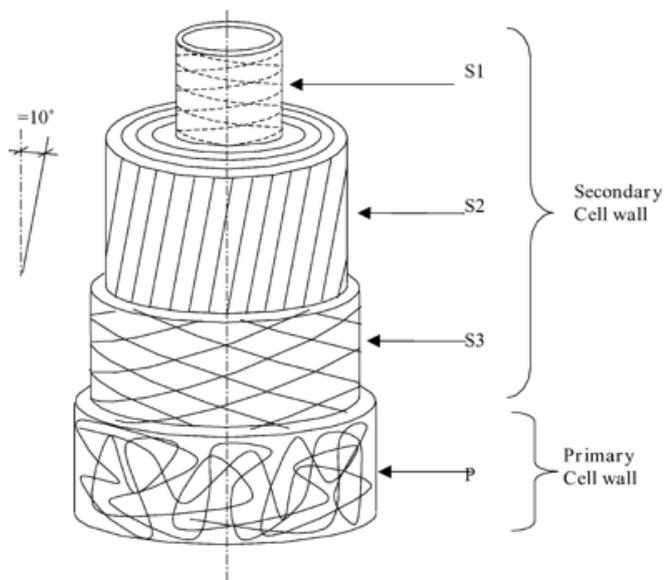
Fig. 1. Schematic diagram of flax fibre architecture (reproduced from [1] by permission of Elsevier Science publishing).
