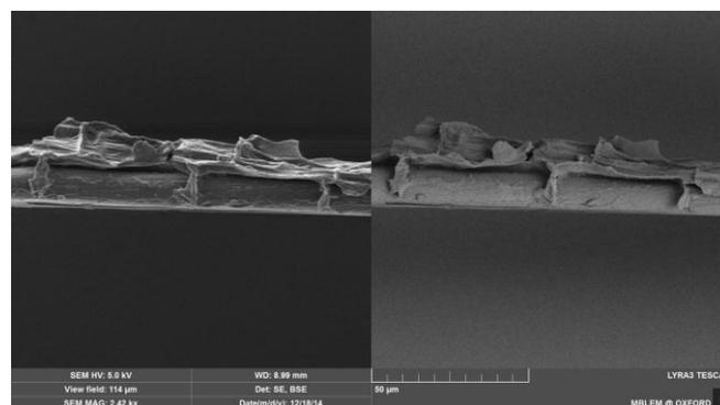
Fig. 3. Moderate magnification SEM images of unretted fibre obtained using secondary electron and back-scattered electron detectors.
