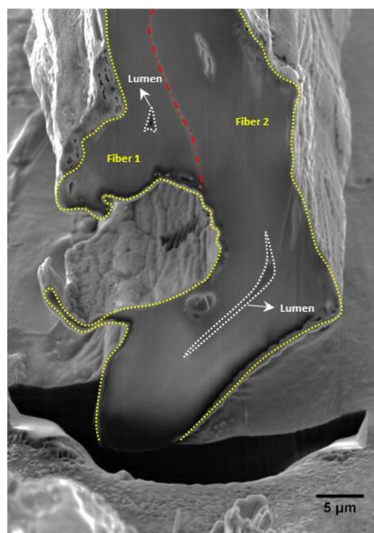
Fig. 6. SEM image of a particular FIB cross-section revealing the major features of a fibre cluster: the outer surface (yellow outer dotted line) and the darker primary wall adjacent to it, the junction between two fibres (red dash-dotted line), and lumen (white dotted lines at fibre core).
