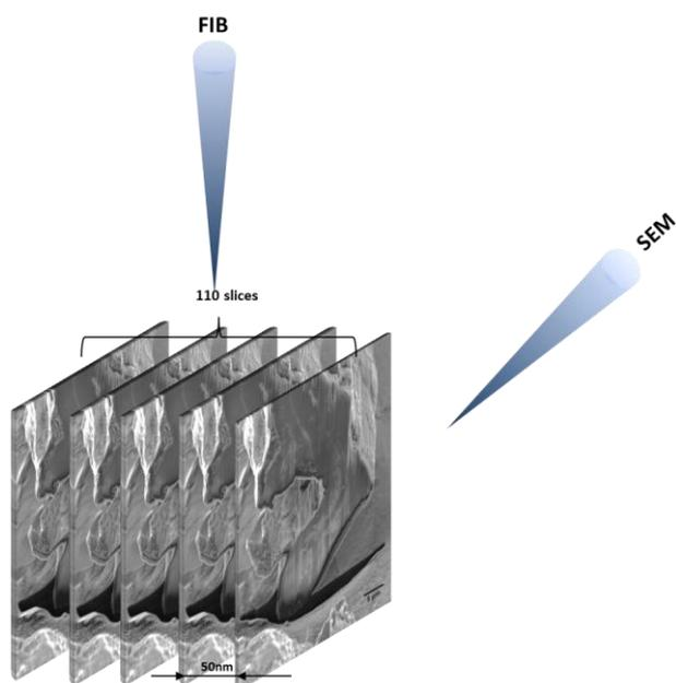
Fig. 5. Illustration of the FIB-SEM configuration for serial sectioning carried out on a cluster of two flax fibres.
