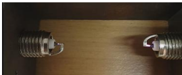
Fig. 8. Example of nature of flame obtained from the sparking plug ignited with multi pulse signal
