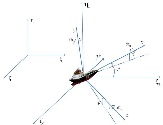
Fig. 1 Main parameters of the vessel
