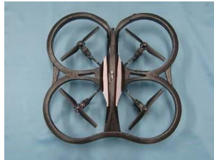
Fig. 12. Multi-rotor drone used as a platform in the present research (AR.Drone2.0. Parrot Corporation)
