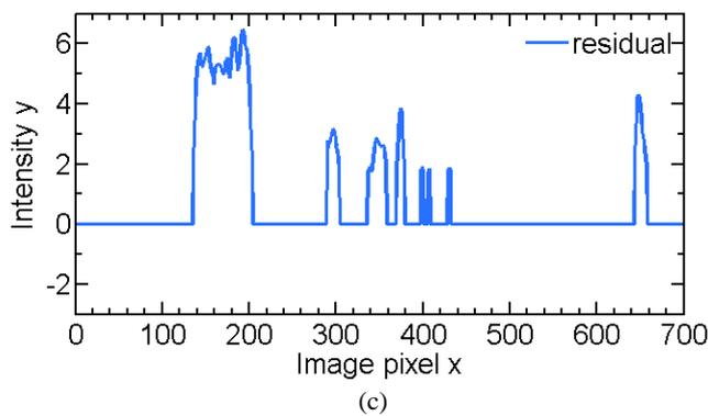
Fig. 3. a) residual data with trend data b) the standard deviation of residual data. c) residual embossed character edges after removed by standard deviation.
