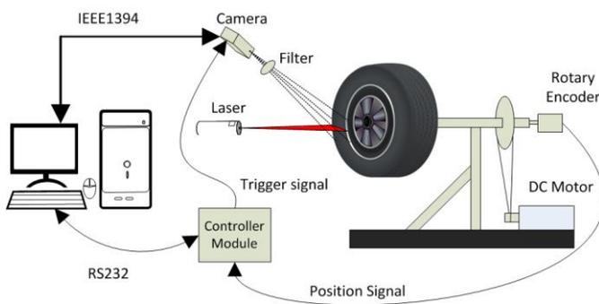
Fig. 2. Tire sidewall surface acquisition system.
