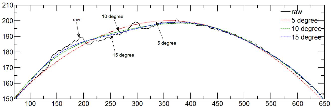
Fig. 4. raw range data curve and 3 varying of power of orthogonal polynomial .
