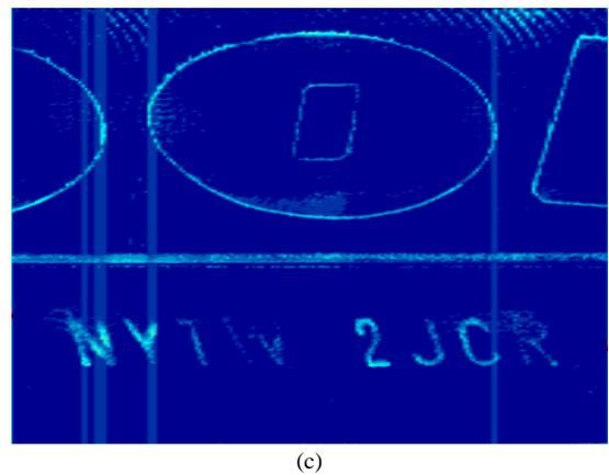
Fig. 5. the 3D surface at DOT code region with different degree of orthogonal polynomials a) degree of 5. b) degree of 10. c) degree of 15.
