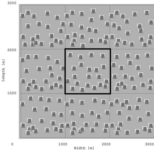
Fig. 3. A snapshot of node distribution in simulations when average number of neighbor nodes is 20
