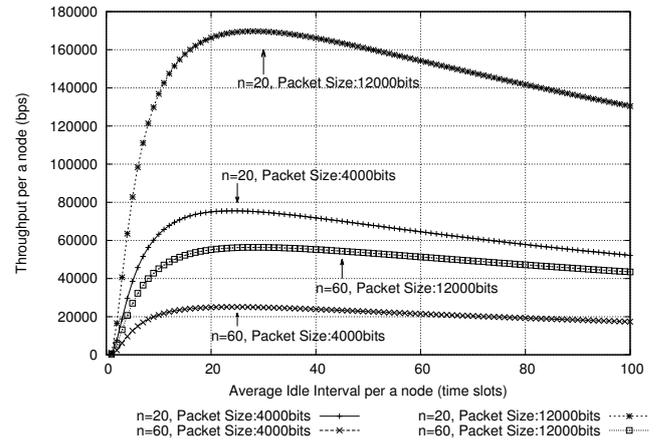
Fig. 2. Throughput with average idle slot interval per a node
