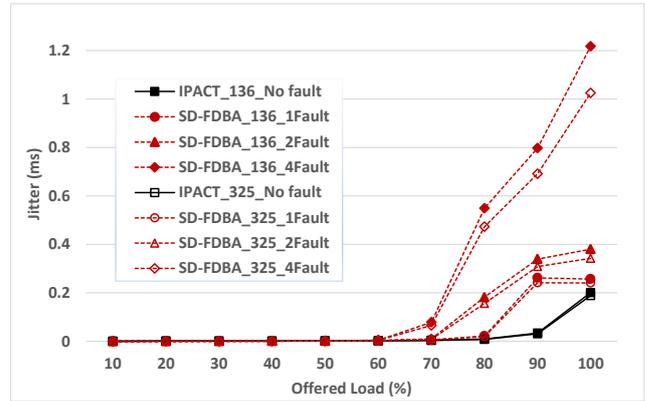
Fig. 5. EF jitter performance comparison of IPACT and SD-FDBA and IPACT in different traffic loads.
