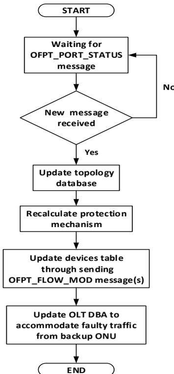
Fig. 3. Detailed operation of the controller in fault condition
