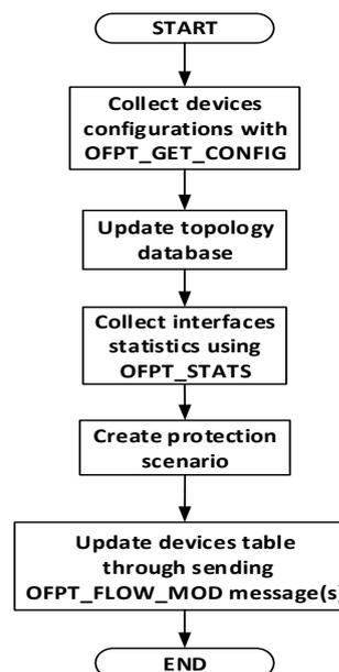
Fig. 2. Detailed operation of the controller in fault protection preparation
