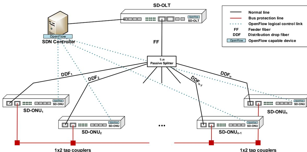
Fig. 1. Proposed software-defined assisted PON multi-DDF protection architecture
