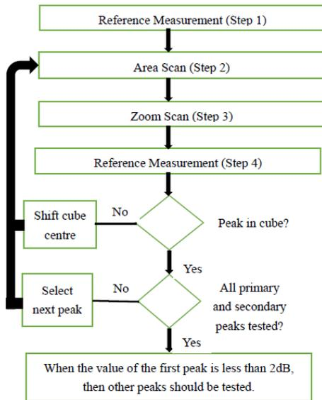
Fig 3. The flow chart of SAR measurement setup
