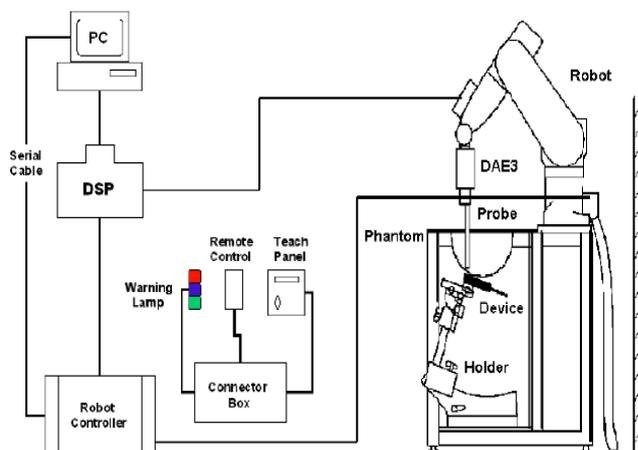
Fig 2. The structure of SAR measurement system by using DASYS-5
