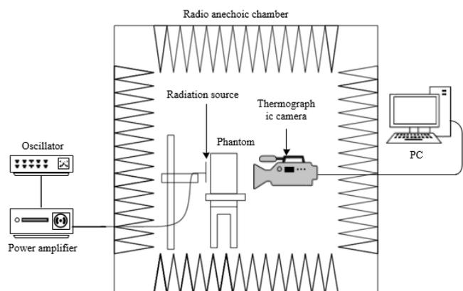
Fig4. SAR measurement system
