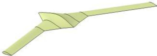
Fig. 4. The CAD model of flying wing aircraft.
