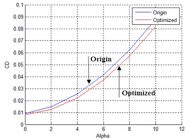
Fig. 12. Drag coefficient comparison of UAV.
