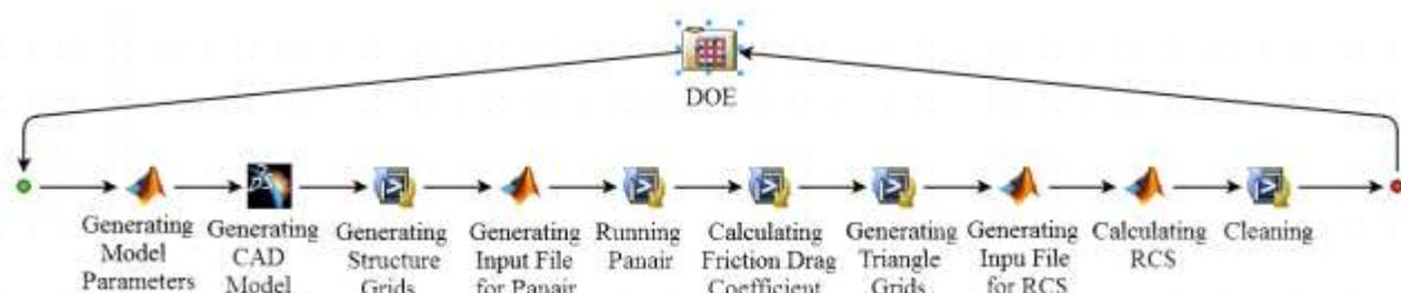
Fig. 5. DOE Flowchart of UAV.
