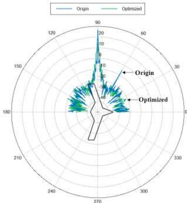
Fig. 14. Distribution comparison of UAV RCS.
