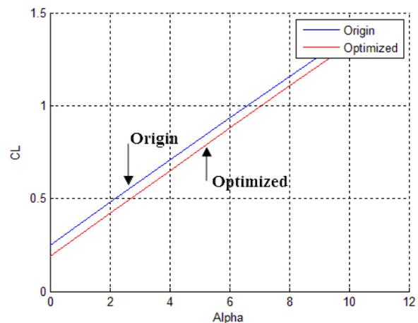
Fig. 13. Lift coefficient comparison of UAV.
