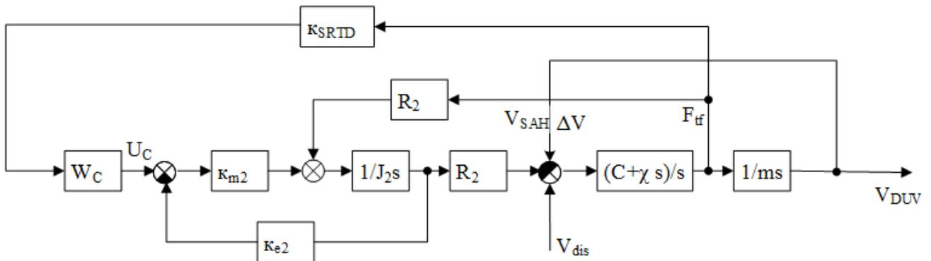
Fig. 3. Blok diagram of position stabilization systems of a descent underwater vehicle with the sensor of rope tension deviation
