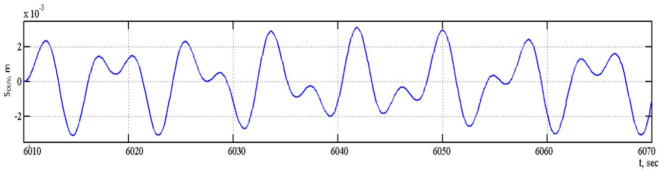
Fig. 8. Variation curves in the vertical movement stabilization mode of the descent underwater vehicle with the sensor of rope tension deviation and the measuring
