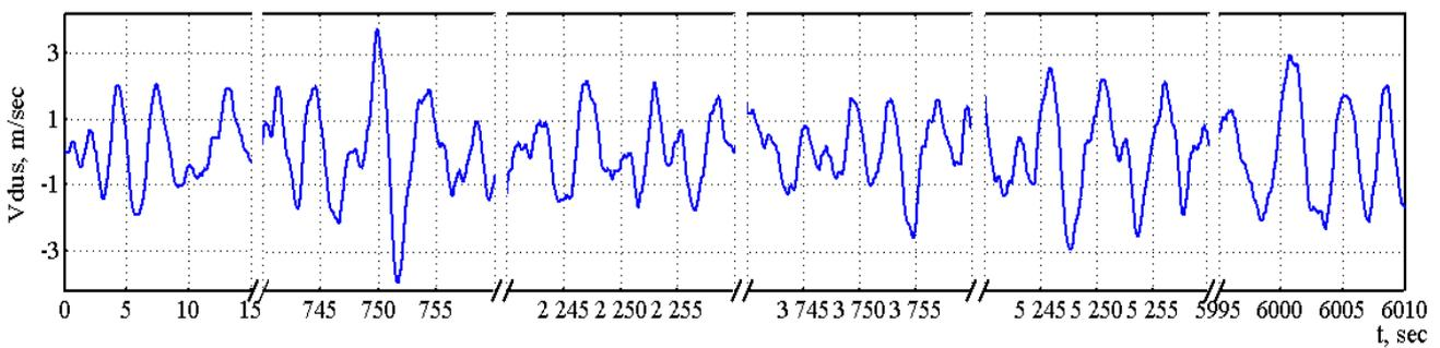
Fig.5. The diagram of the ordinate variation of irregular sea disturbance
