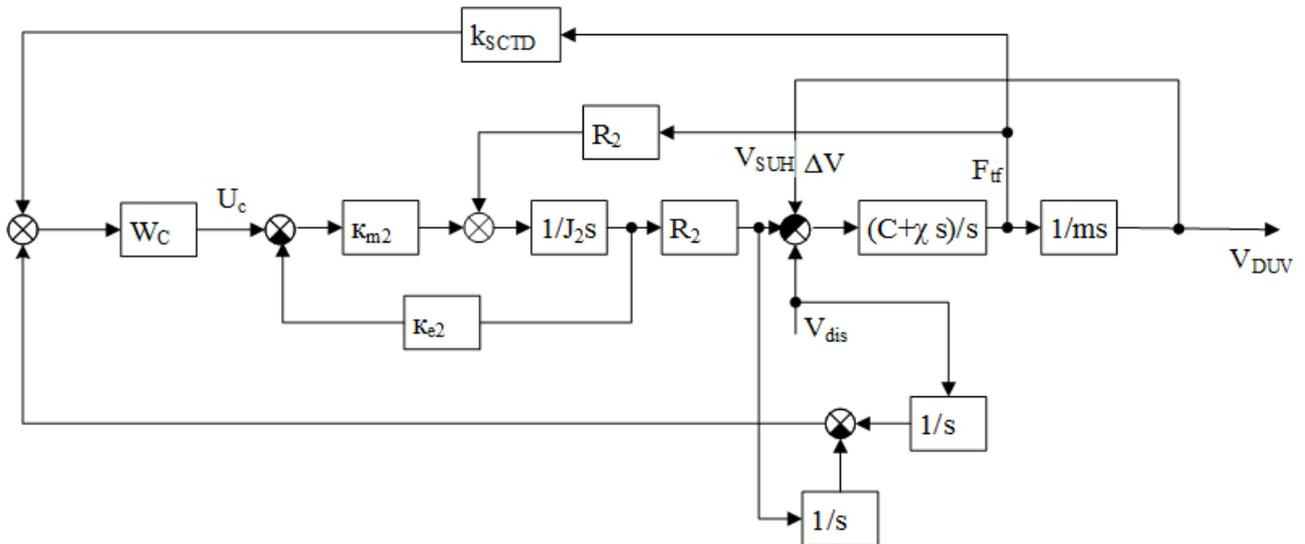
Fig. 4. Blok diagram of position stabilization systems of a descent underwater vehicle with the sensor of rope tension deviation and the measuring
