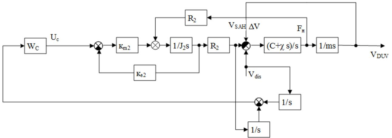
Fig. 2. Blok diagram of position stabilization systems of a descent underwater vehicle with the measuring converter
