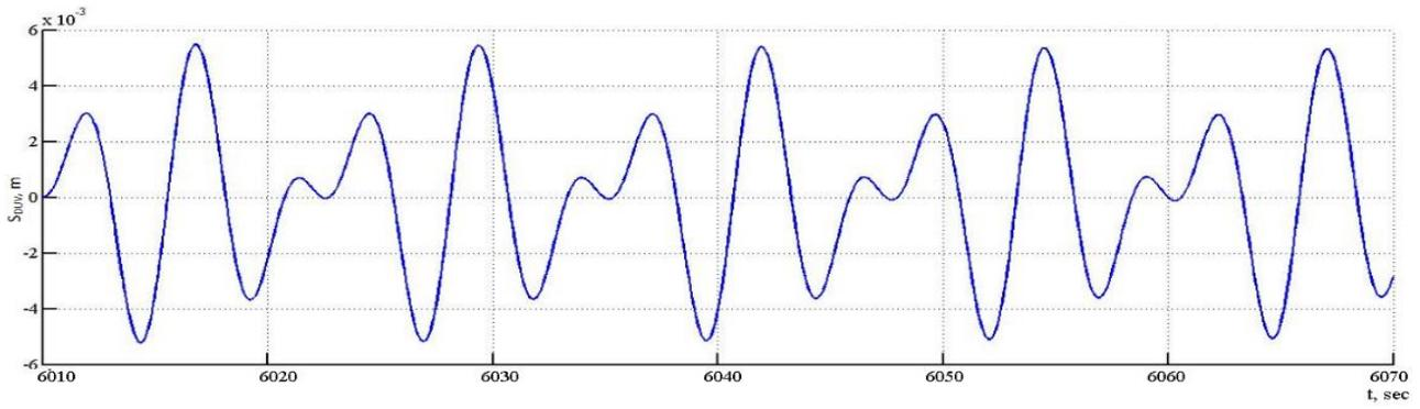
Fig. 6. Vertical movement variation curves of the descent underwater vehicle with the measuring converter
