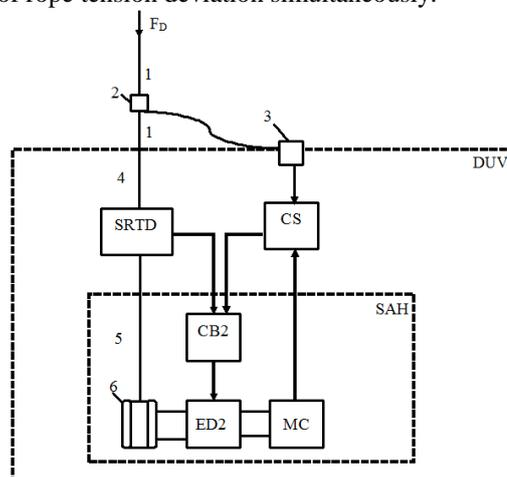
Fig. 1. Stabilization system of a descent submersible vehicle location
