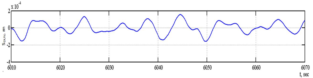
Fig. 7. Vertical movement variation curves of the descent underwater vehicle with the sensor of rope tension deviation
