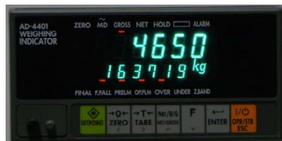
Fig. 19. Weighing data on local readout of the AD-4401 indicator.
