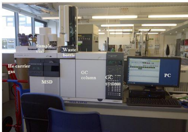
Fig 2. Agilent technologies 7890B autosampler Gas chromatography (GC) system coupled with Agilent technologies 5977A mass spectrometry detector (MSD) at the Centre for Process Integration and Membrane Technology
