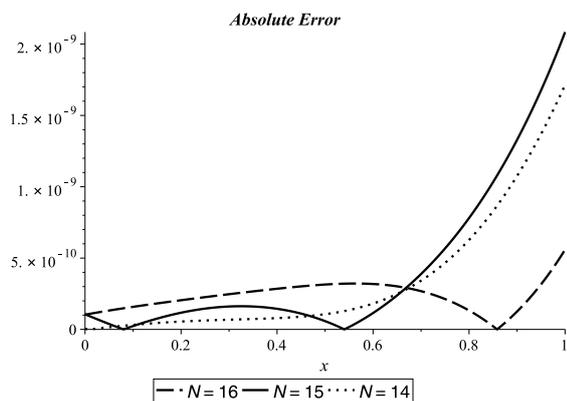
Fig. 2. Graph of absolute error of the static deflection of the beam for Ex.1
