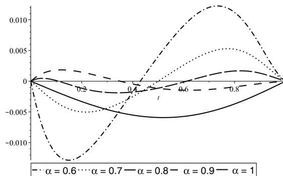
Fig. 3. Graphical solutions for deflection of the static beam for fractional order  $\alpha = 0.6, 0.7, 0.8, 0.9, 1$
