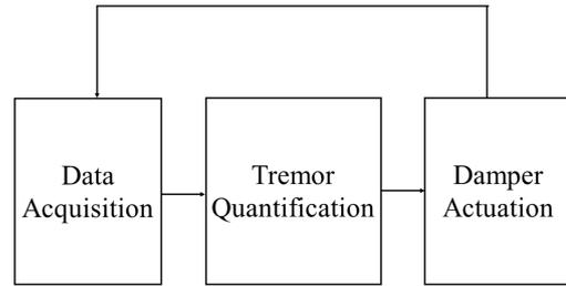
Fig. 5. Software Implementation Block Diagram. The software implementation was divided into three parts: a) data acquisition, b) tremor extraction, and c) actuation.
