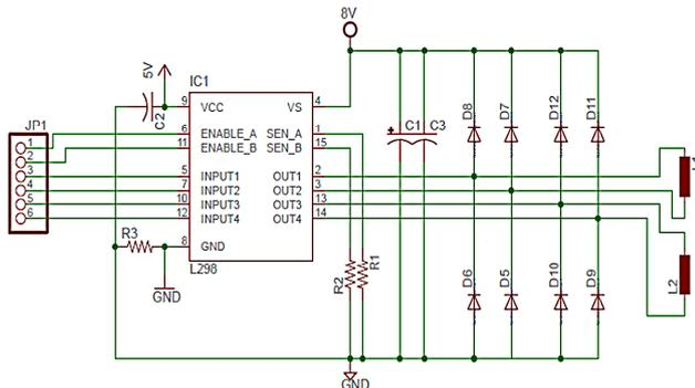
Fig. 3. Dual H-Bridge Driver Schematic. An L298 dual H-bridge was used to drive the pair of electromagnetic coils (i.e. right and left). The microcontroller would be sending TTL signals on the pair of coils on the opposite direction of the detected motion, and with frequency dependent on the frequency of the hand tremors.
