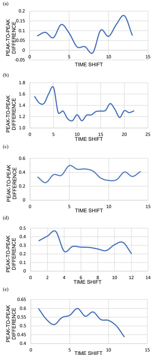
Fig. 9. Time-Shifted Peak Difference. (a) Tremor signal 1 at 5Hz with amplitude 5.10°, first peak alignment is at time shift 11. (b) Tremor signal 2 at 3Hz with amplitude 11.07°, first peak alignment is at time shift 4. (c) Tremor signal 3 at 4.5Hz with amplitude 3.56°, first peak alignment is at time shift 12. (d) Tremor signal 4 at 5.5Hz with amplitude 6.29°, first peak alignment is at time shift 10. (e) Tremor Signal 5 at 5Hz with amplitude 2.41°, first peak alignment is at time shift 11.
