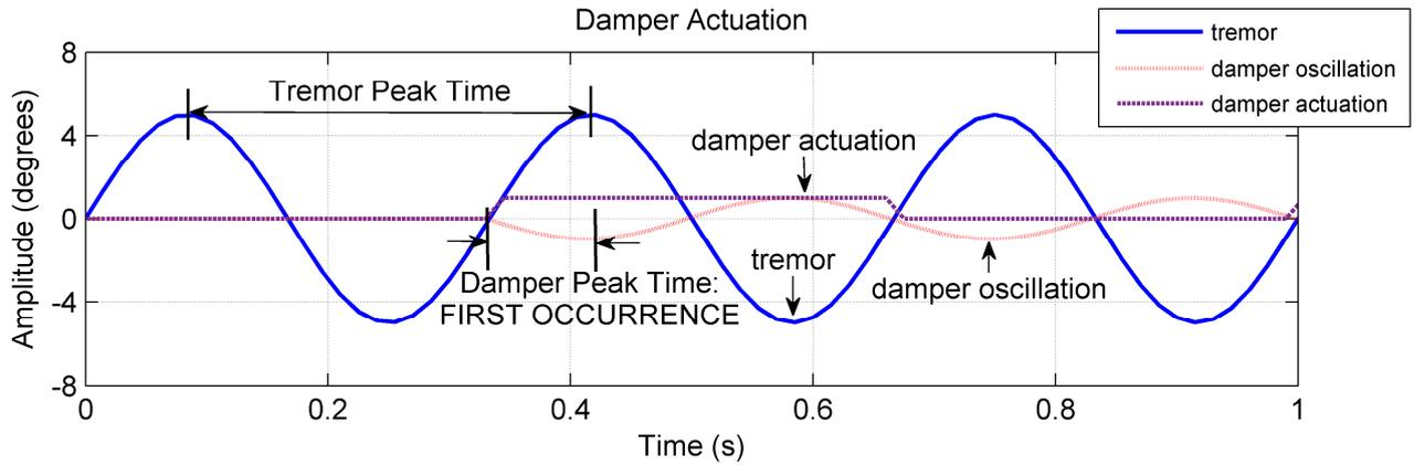
Fig. 7. Theoretical Peak Reading. This is the ideal case scenario for actuation. Tremor Peak Time is the time difference between the occurrence of the first two peaks. The Damper Peak is the time when the oscillation caused by the system first peaks.
