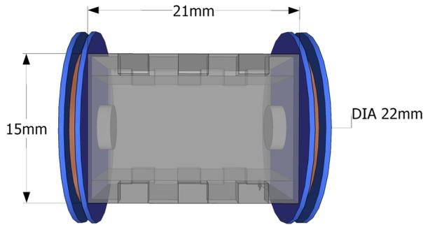
Fig. 2. Mounting case model. The mounting case is 21mm x 21mm x 15mm, laser-cut from a 2mm thick acrylic sheet. The two solenoids were attached to the left and right of the mounting case.
