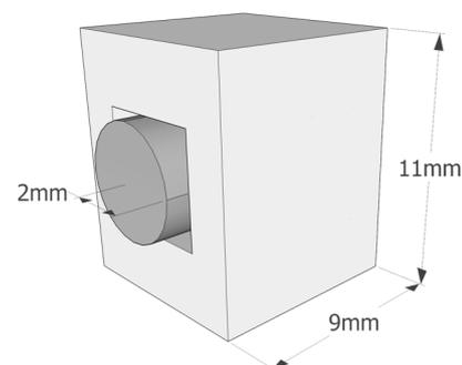
Fig. 1. Mass damper model. The mass damper was 3D-printed and attached on the left and right faces were neodymium magnets (NdFeb D5mm x 2mm N42) with  $B = 0.507$  T, both North exposed. It was restricted to move along a single axis (y-axis).
