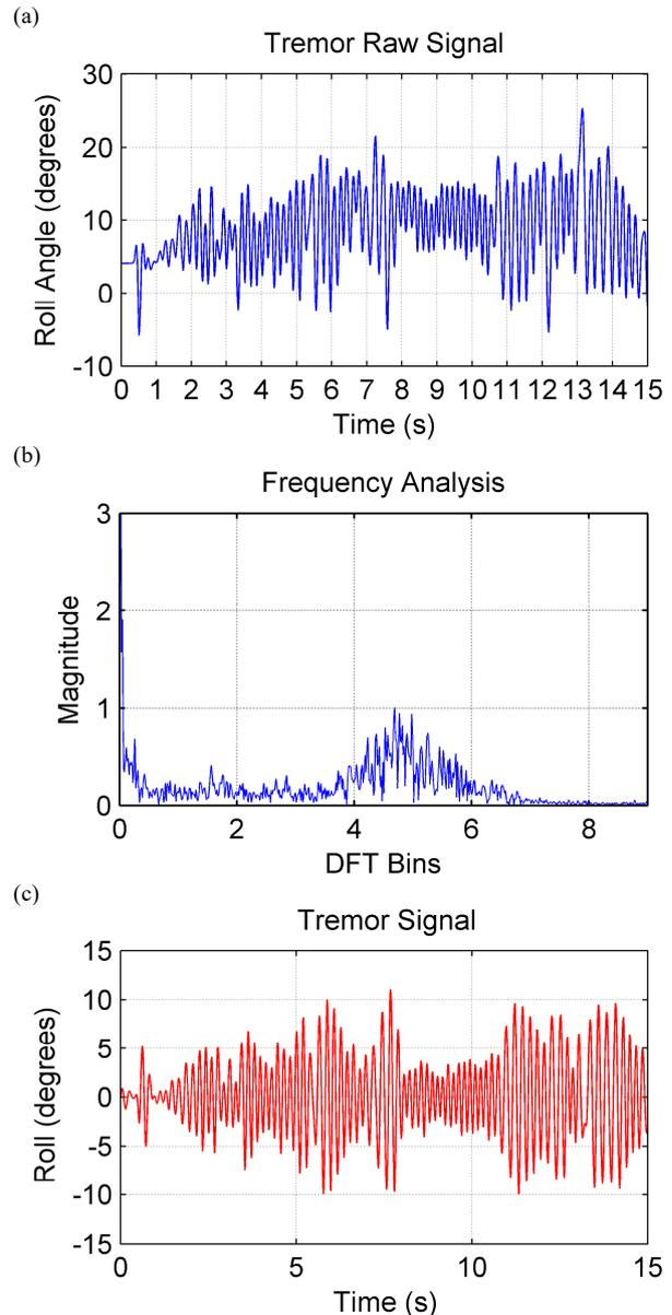
Fig. 8. Sample Tremor Signal 1 at 5Hz. (a) Raw signal from hand raised shoulder-level. (c) Spectral peak at 5Hz. (d) Extracted tremor signal.
