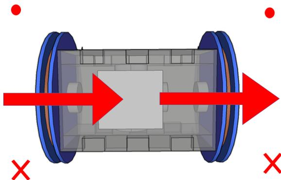
Fig. 4. Actuation Direction. • denotes that the current goes out of the page; while X denotes that the current goes into the page; and → denotes the direction of the magnetic field.
