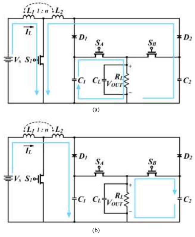
Fig. 3. Topologies for Phase (a) I and  $S_A$ : SPWM-ON, (b) II and  $S_B$ : SPWM-ON.
