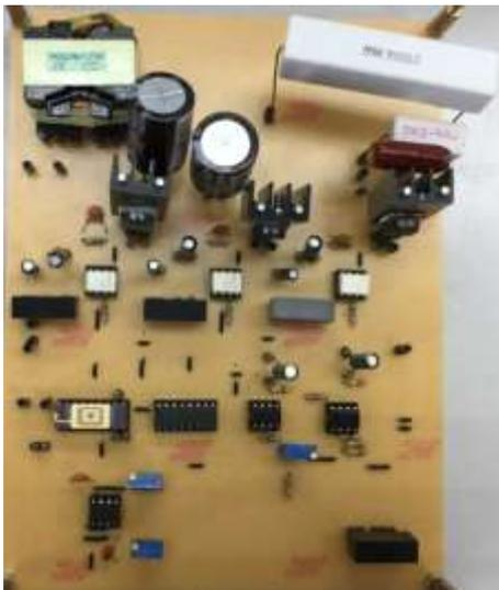
Fig. 6. Prototype circuit of closed-loop SCII.
