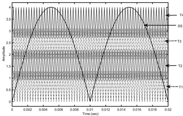
Fig. 5: Carrier signal alignment in CO SPWM
