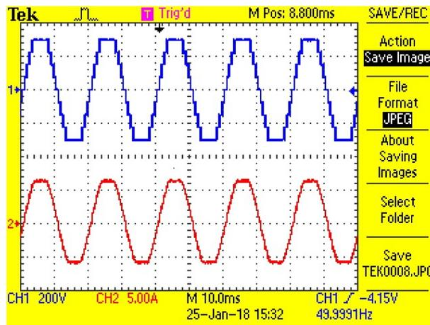
Fig. 10: HIL results of output voltage and current for RL load and  $m_a = 0.8$
