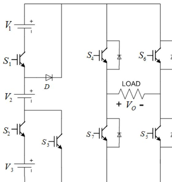
Fig. 1: Circuit diagram of proposed multilevel inverter
