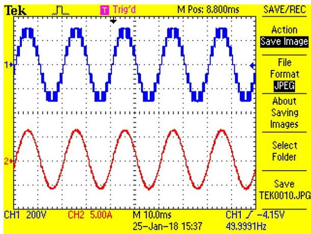
Fig. 8: HIL results of output voltage and current for RL load and  $m_a = 1$
