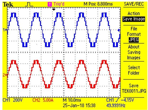
Fig. 6: HIL results of output voltage and current for R load and  $m_a = 1$
