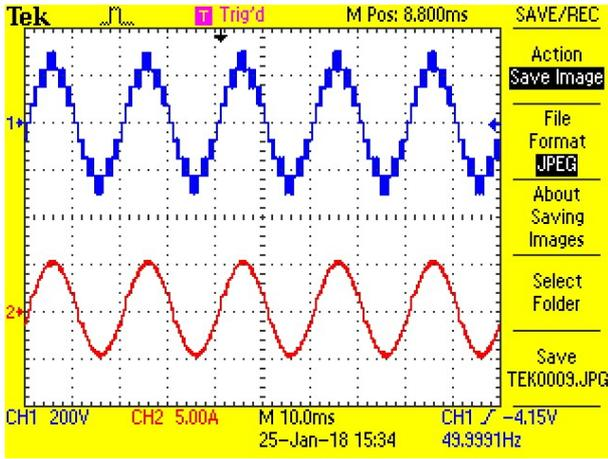
Fig. 12: HIL results of output voltage and current for RL load and  $m_a = 1.2$
