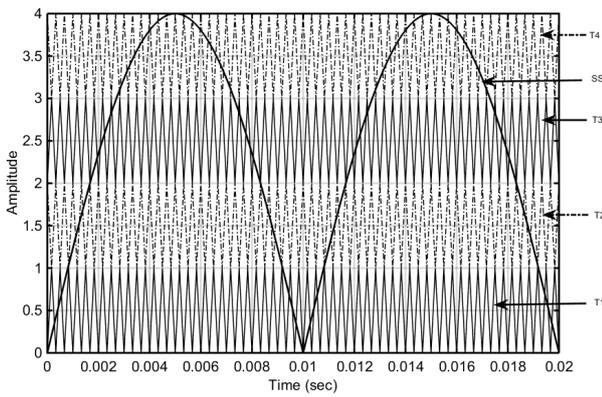
Fig. 4: Carrier signal alignment in APOD SPWM
