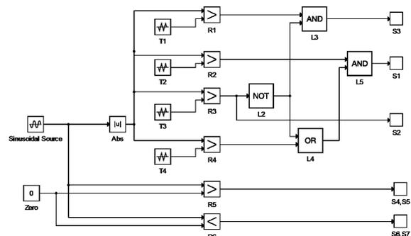
Fig. 3: Control block generating gate pulses using SPWM technique
