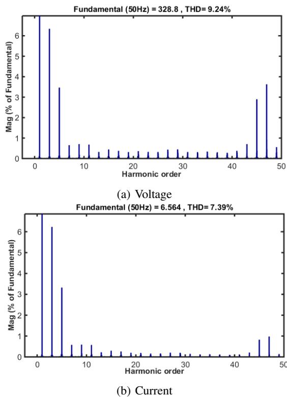
Fig. 13: FFT analysis for RL load and  $m_a = 1.2$
