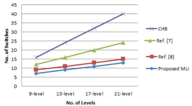
Fig. 2: Comparison between number of switches used in various inverter topologies
