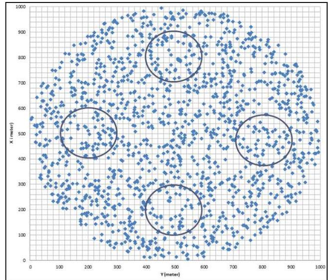
Fig. 2. Placements of macrocell, picocells and UEs
