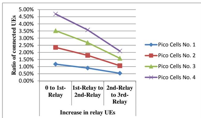
Fig. 7. Change in connected UEs as relays increase for 300 Requesting UEs
