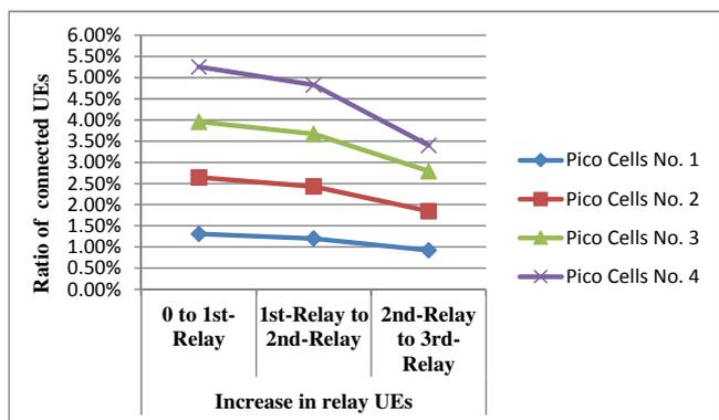
Fig. 6. Change in connected UEs as relays increase for 150 Requesting UEs
