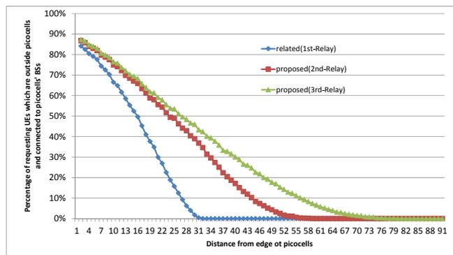
Fig. 10. Percentage of requesting UEs which are outside picocells and connected to BSs of picocells for 300 requesting UEs and 4 picocells
