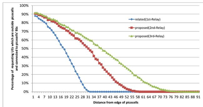
Fig. 9. Percentage of requesting UEs which are outside picocells and connected to BSs of picocells for 150 requesting UEs and 4 picocells
