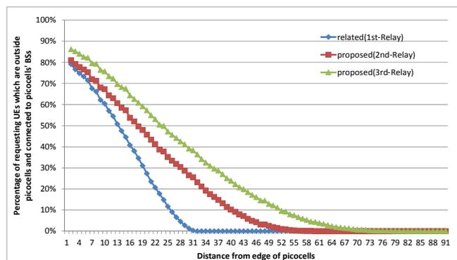
Fig. 11. Percentage of requesting UEs which are outside picocells and connected to BSs of picocells for 450 requesting UEs and 4 picocells
