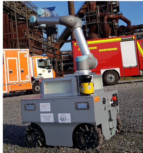
Figure 1. Mobile manipulator OmniMan : UR5 robotic arm on a Mecanum wheeled mobile platform
