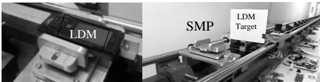
Fig. 3. The LDM is the unit under calibration (left), and the SMP is shown on the right
