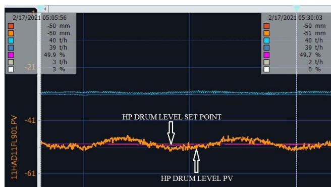
Fig. 6 Water level control of high pressure drum boiler during Off-Peak Mode Operation using PID control parameters set 1
