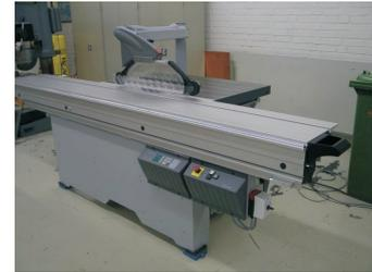
Figure 1: Picture of a sliding table saw.
