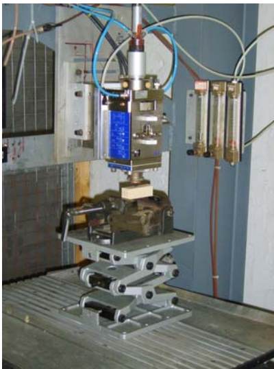
Figure 1. YLR-1000-SM Ytterbium-doped fibre laser system employed with the cutting set up.
