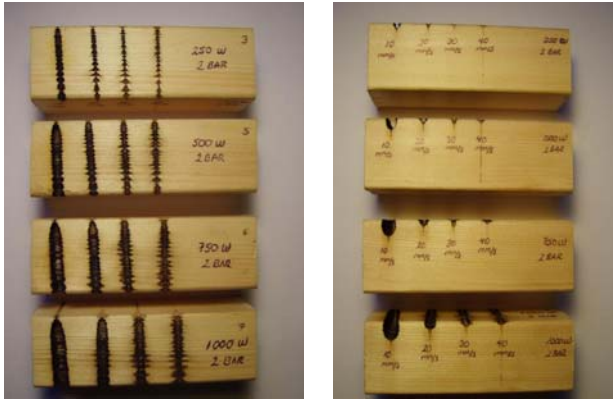
Figure 2. Top and side view of the samples cut by fibre laser beam in the radial direction.
