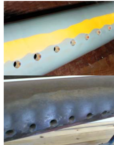
Fig. 9 Model and Full Scale Sparge Pipe Wear Patterns
