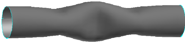
Fig. 3. The buckling patter of a (18,0) CNT of 8.7 nm length using higher order gradient theory.
