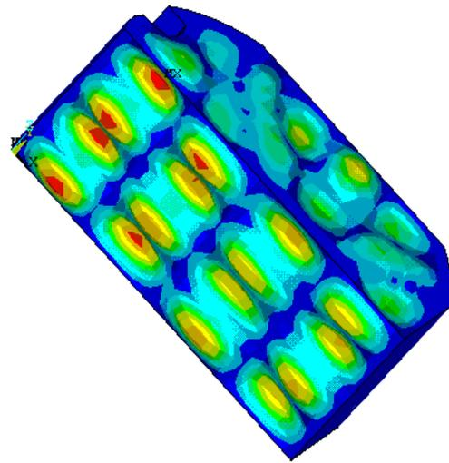
**Figure 6** Structural displacement pattern for coupled structural mode at frequency  $f=57.33$  Hz.
