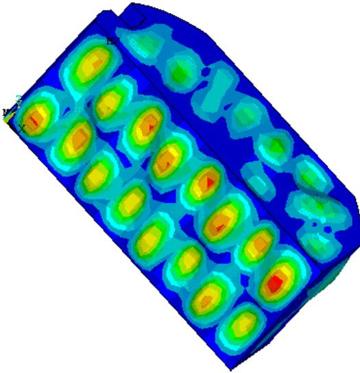
**Figure 4** Structural displacement pattern for coupled “combined” mode at frequency  $f=58.26$  Hz.
