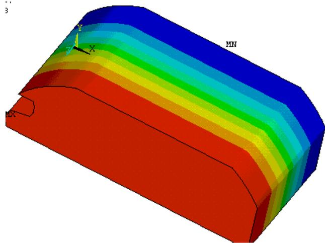
**Figure 3** Second rigid-walled acoustic mode of passenger compartment at frequency  $f_a=103.1.3$  Hz.
