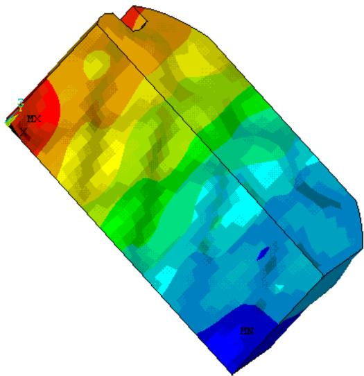
**Figure 5** Pressure pattern for coupled “combined” mode at frequency  $f=58.26$  Hz.
