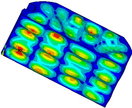
**Figure 8** In-vacuo structural vibration mode of passenger compartment at frequency  $f_s=57.89\text{Hz}$ .
