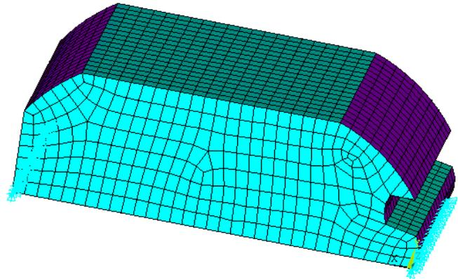
Figure 1 FE model of vehicle compartment.
