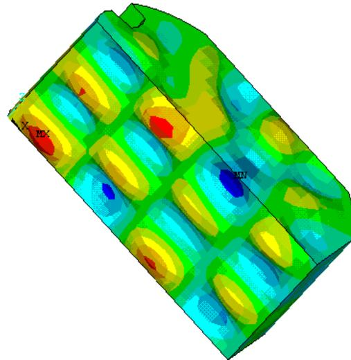
**Figure 7** Pressure pattern for coupled structural mode at frequency  $f=57.33$  Hz.
