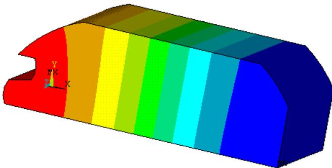
**Figure 2** First rigid-walled acoustic mode of passenger compartment at frequency  $f_a=57.3$  Hz.
