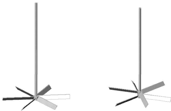
Figure 2: (a)Simple blade (b)Complex blade configuration
