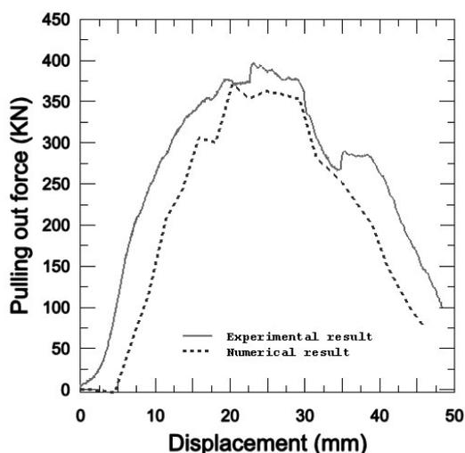
Fig. 2. Pulling force versus displacement of a porcine bone and calf tendon fixed at one end.
