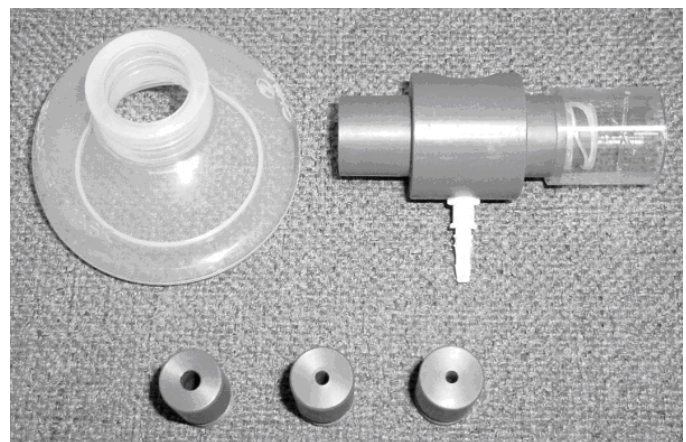
Figure 2: Customized apparatus used in this study to simulate increased breathing efforts; facemask, IRL and an adaptor including a unidirectional airflow valve, an air pressure measure outlet and mechanical guard
