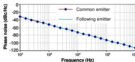
Fig. 8 Phase noise due to noise sources of cross-coupled transistors for the two buffers configurations
