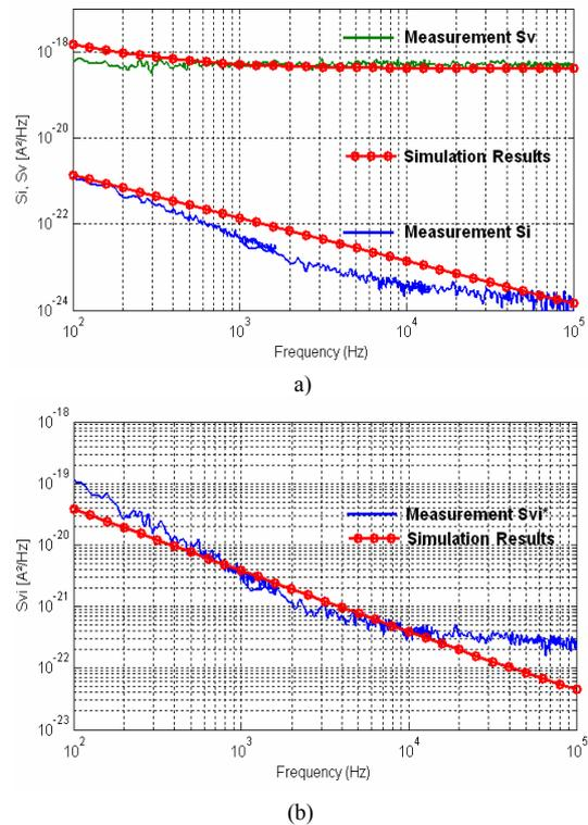
Fig. 5 (a)  $S_V$  and  $S_I$  spectra and (b) their cross-spectrum  $S_{VI}^*$ , simulated and measured. The spectra obtained with the HBT, respectively, biased at  $I_B=1 \mu\text{A}$ ,  $I_C=1.3 \text{ mA}$ . The HBT under test features an emitter area of  $0.17 \mu\text{m} \times 6.2 \mu\text{m}$
