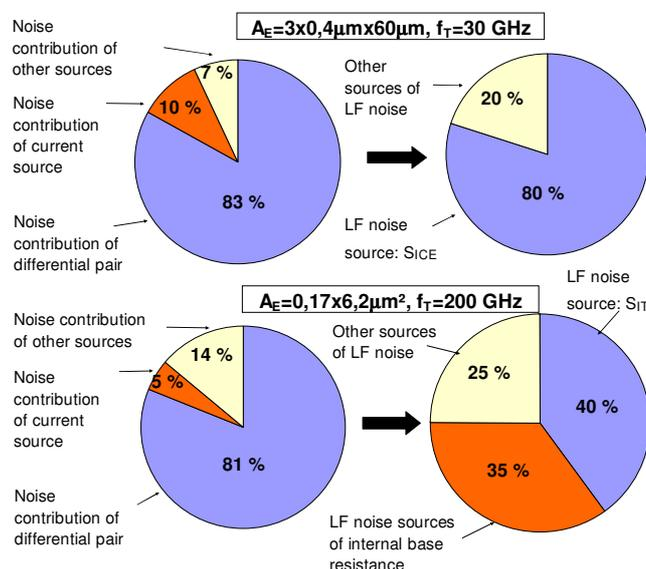
Fig. 10 Phase noise due to noise sources of cross-coupled transistors for the two buffers configurations
