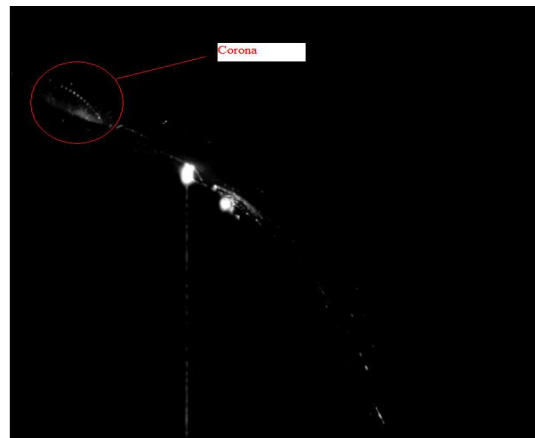
Figure 2.5 Corona structure indicating wet surface
