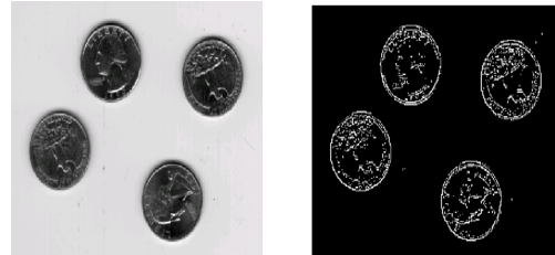
Fig. 3. (a) Original Coins Image; (b) After Averaging and Edge Detection Templates by adapting RK-Embedded Centroidal Mean.
