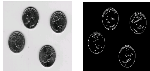
Fig. 5. (a) Original Coins Image; (b) After Averaging and Edge Detection Templates by adapting RK-Embedded Contra-Harmonic Mean.
