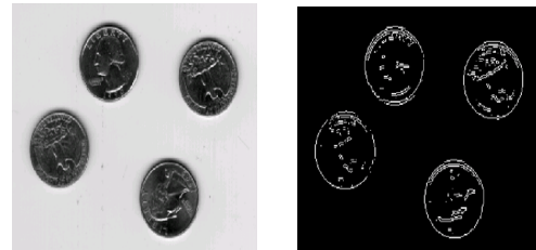
Fig. 4. (a) Original Coins Image; (b) After Averaging and Edge Detection Templates by adapting RK-Embedded Harmonic Mean.
