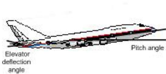
Figure 1: Elevator deflection angle and pitch angle.
