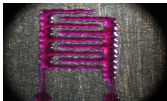
Fig. 5. Test structure printed at highest speed.
