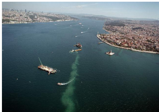
Figure 8: Turbidity plume due to dredging in the Istanbul Strait
