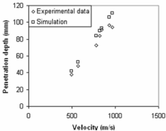
Fig.4 Penetration depth versus velocity for 6061-T6511 aluminium alloy by spherical nose projectile (experimental data are from [4])
