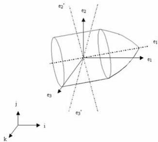
Fig. 1 Reference frame for projectile motion
