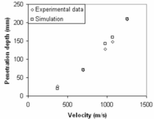
Fig.6 Penetration depth versus velocity for 7075-T651 aluminium alloy by ogive nose projectile (experimental data are from [5])
