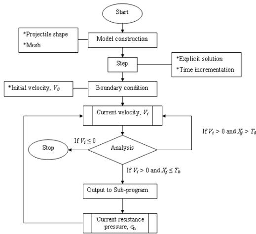
Fig.3 Flow chart of communication between core and sub programs
