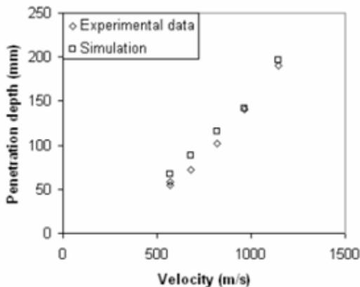
Fig.5 Penetration depth versus velocity for 6061-T6511 aluminium alloy by ogive nose projectile (experimental data are from [5])
