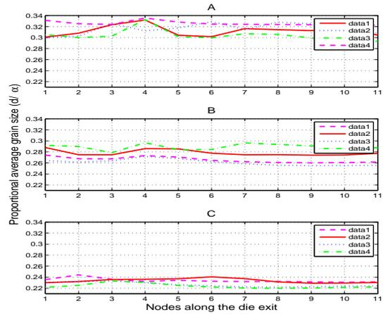
Figure 2: Grain size variation along the die exit ( $d/\alpha$ ) (A) when  $v = 6.3 \text{ mm/s}$ ,  $T_{D_0} = 450^\circ\text{C}$ ,  $T_{B_0} = 500^\circ\text{C}$ , (B) when  $v = 25 \text{ mm/s}$ ,  $T_{D_0} = 450^\circ\text{C}$ ,  $T_{B_0} = 500^\circ\text{C}$ , (C) when  $v = 25 \text{ mm/s}$ ,  $T_{D_0} = 400^\circ\text{C}$ ,  $T_{B_0} = 450^\circ\text{C}$ .
