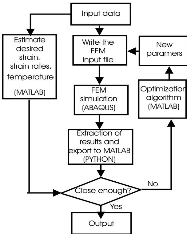
Figure 1: Illustration of design process.
