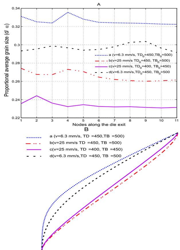
Figure 3: Grain size variation along the die exit ( $d/\alpha$ ):(A) Optimal vales with different process conditions, (B) Optimal die shape with different process conditions .
