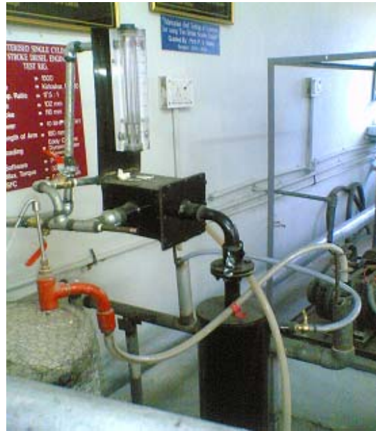
Figure (VI):- Exhaust gas recirculation set up
