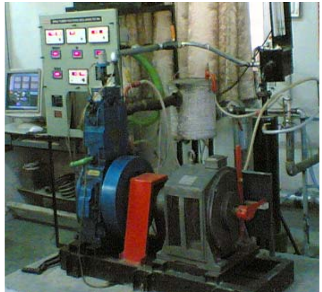
Figure (VII):- Exhaust gas recirculation set up coupled with engine
