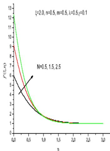
Figure 13: Velocity distribution for different values of sustantation parameter  $N$ .
