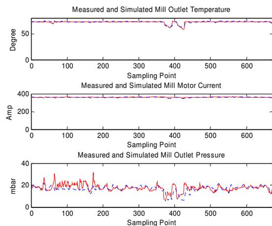
Figure 8 measured (solid lines) and simulated (broken lines) using PSO
