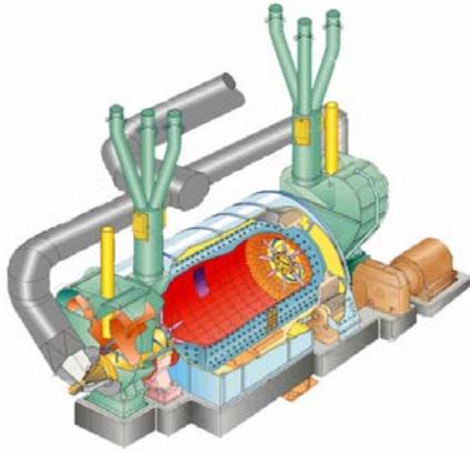
Figure 2 Tube Ball Mill Structure
