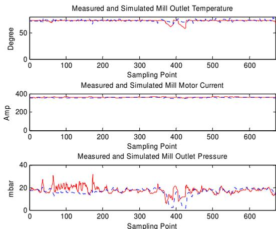
Figure 10 measured (solid lines) and simulated (broken lines) using GA
