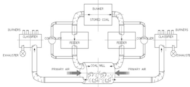
Figure 1 Tube Ball Mill Principle of Operation
