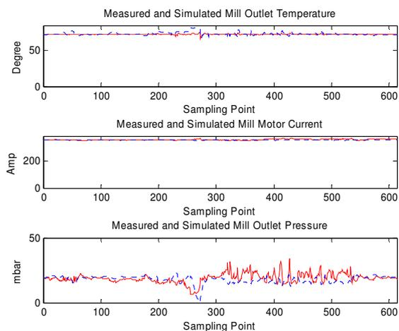
Figure 11 measured and simulated results using the initial model
