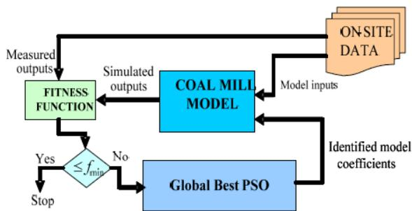
Figure 6 Schematic of the model's coefficients identification
