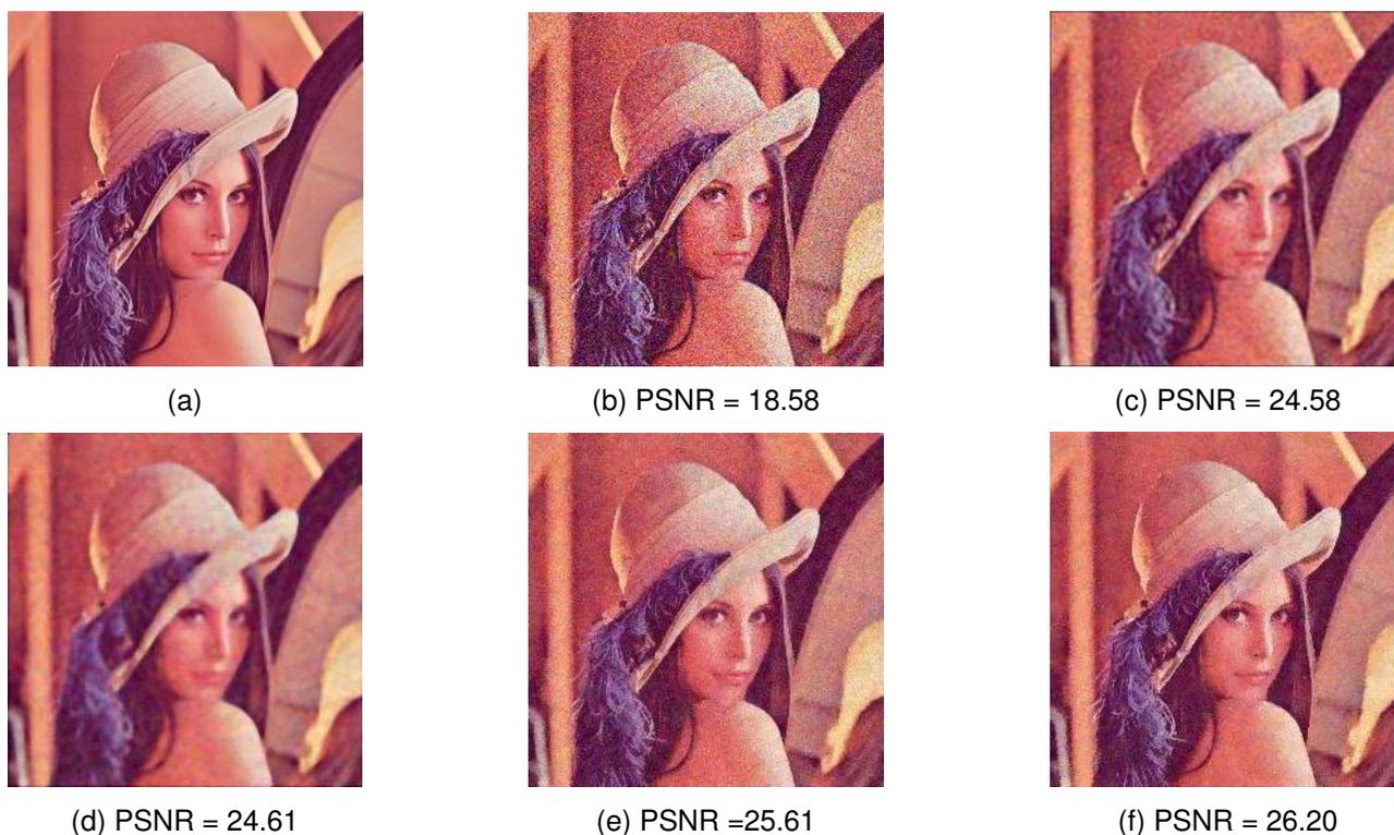
Fig. 2. (a) Original Lena image (256x256) (b) Noisy image (Gaussian noise,  $\sigma = 30$ ) (c) After applying Mean filter (3x3 window) (d) After applying Median filter (5x5 window) (e) After applying Fuzzy filter of [24] with K=3 (7x7 window) and L=2 (5x5 window) (f) After applying Proposed Fuzzy filter with K=3 (7x7 window) and L=2 (5x5 window)
