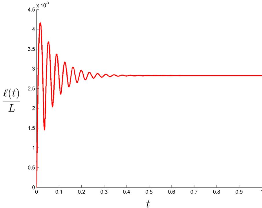
Figure 4: Water meniscus oscillations inside a close-end capillary for  $\lambda = 1$ , and  $R = 0.005$  m.
