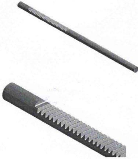
Figure 1: Car steering rack.
