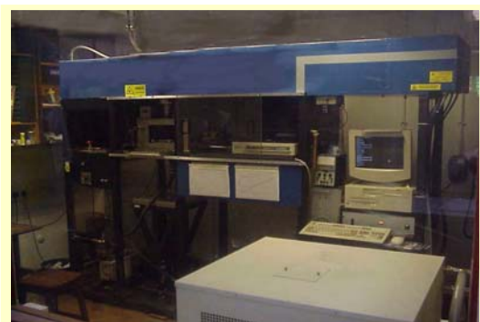
Fig. 4 CO 2 SLS experimental machine used to fabricate test specimen
