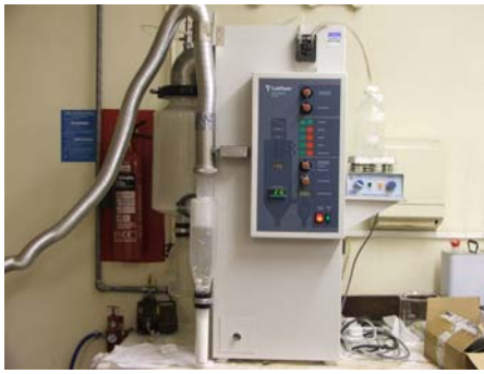
Fig. 3 SD-05 spray dryer machine used in production of powder
