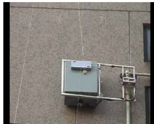
(f) The robot stopped when reaching the end of the gas pipe and waited for the instruction to come back.
