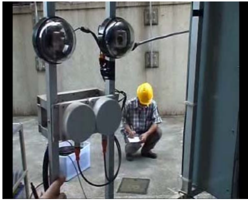
(a) The two cameras and the two proximity sensors
