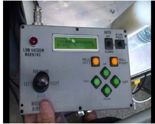
(b) The operator control console
