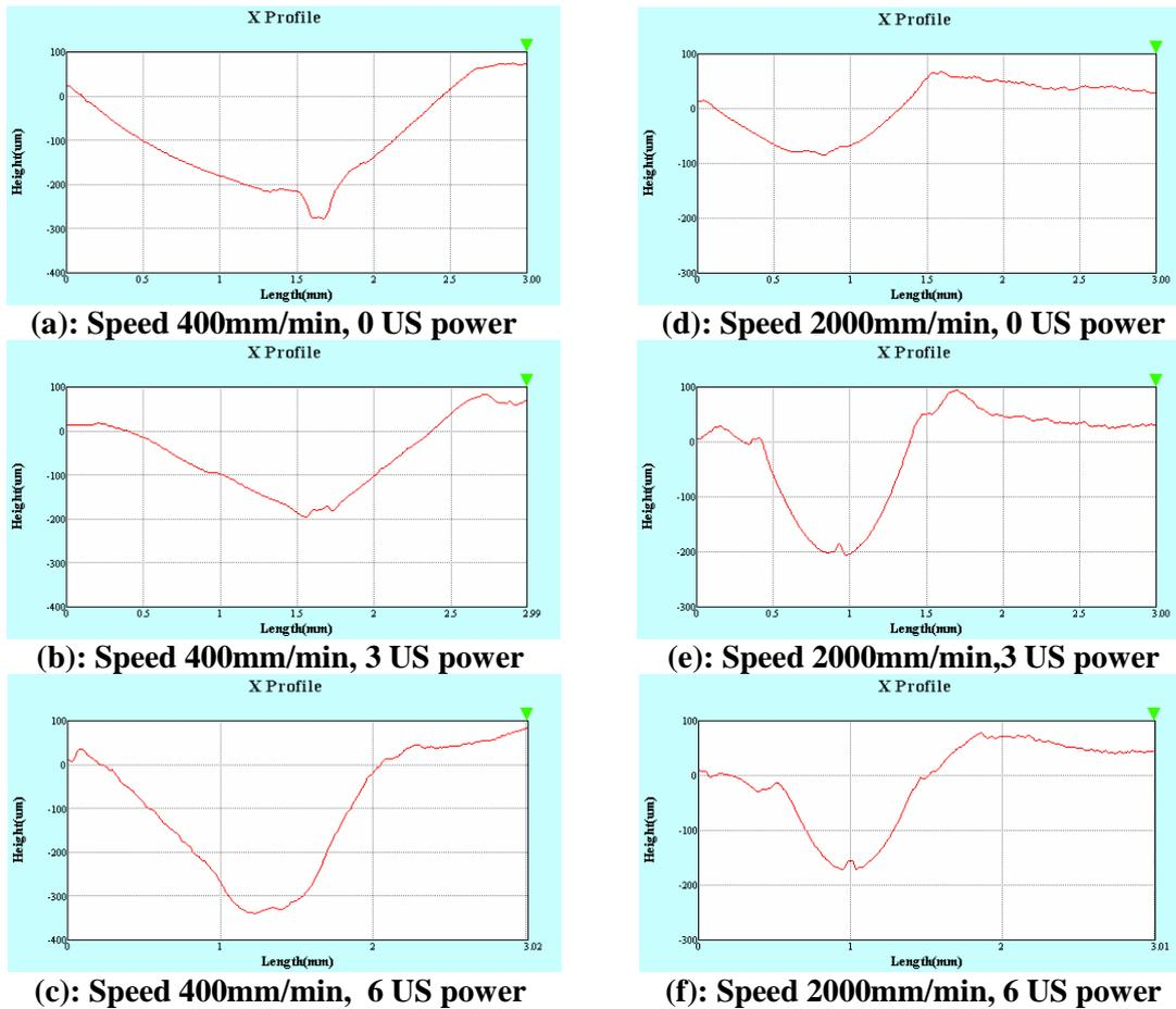
**Fig 4: 2D Profile along Center of Weld**
