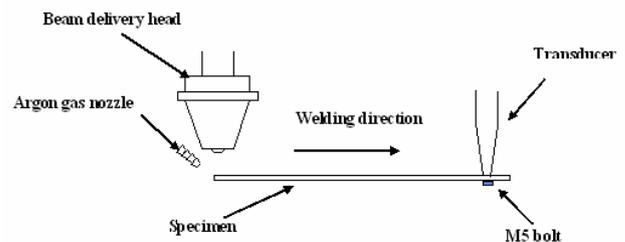
Fig 1: Set Up for the Laser Welding
