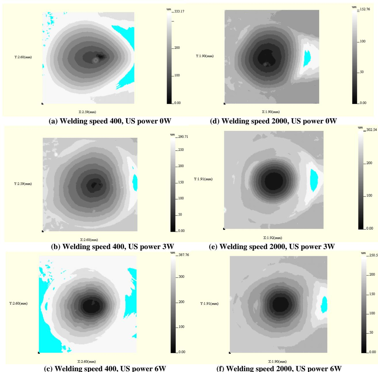
**Fig 2: 2D Weld Bead Geometry Showing Material Distribution**
