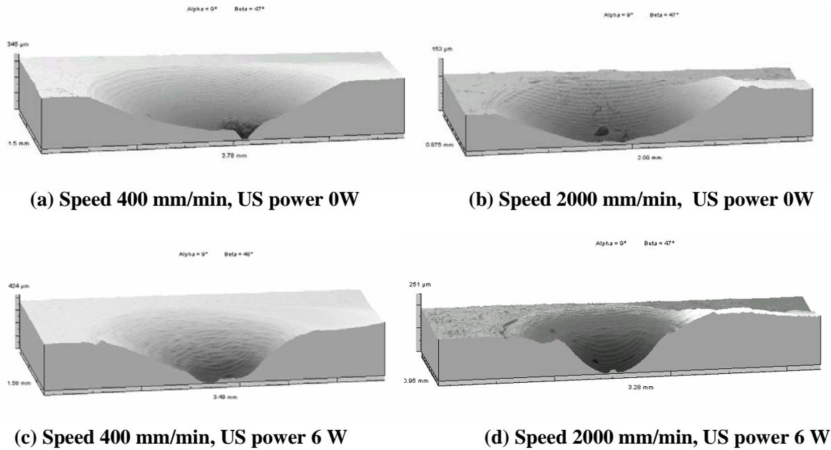
**Fig 3: 3D Section Through Weld Bead**
