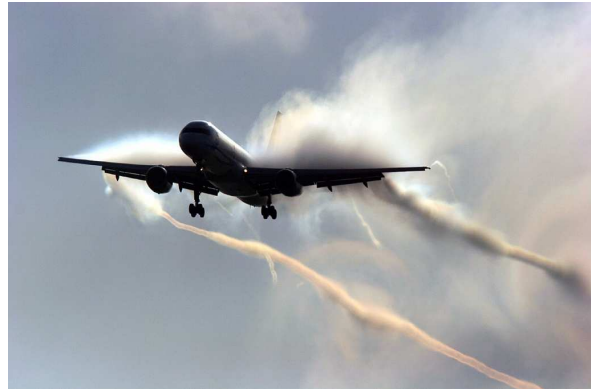
Fig. 1 Aircraft Wake Vortex
