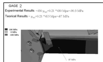
Fig. 14: Numerical - experimental analysis for gage 2
