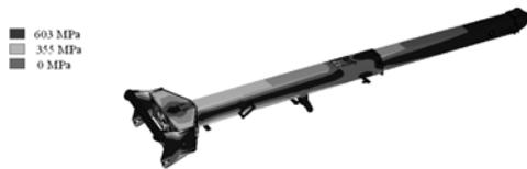
Fig. 10: Von Mises Stress for the additional load case 1
