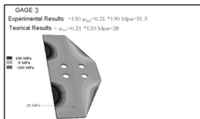
Fig. 15: Numerical - experimental analysis for gage 3
