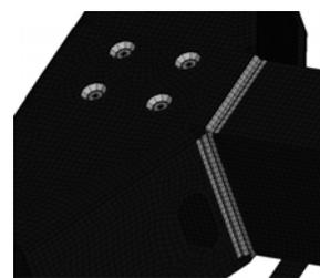
Fig. 5: Butt weld zone
