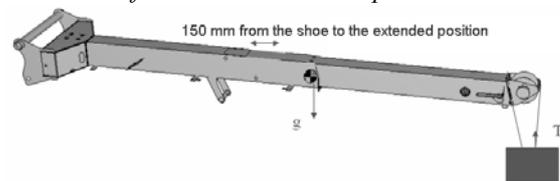
Fig. 9: Additional load case 3 for a telescopic crane jib.
