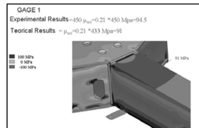
Fig. 13: Numerical - experimental analysis for gage 1
