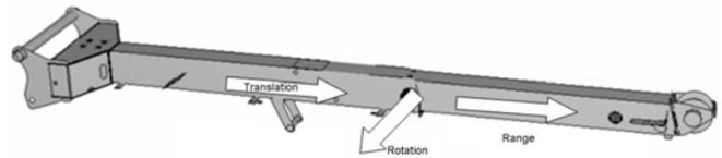
Figure 1: Movements in a telescopic crane jib
