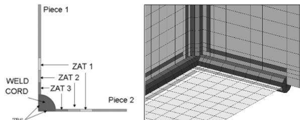
Fig. 3 y 4: Butt weld zone. Corner weld model with ZBS y HAZs
