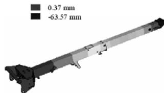
Fig.11: Vertical displacements for the adicional load case 3
