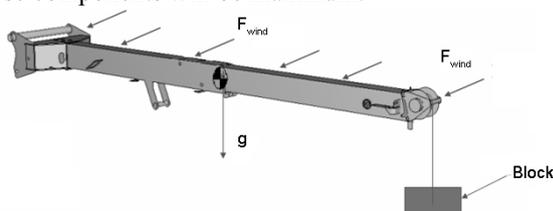
Fig. 6: Load Case 2 for a telescopic crane jib
