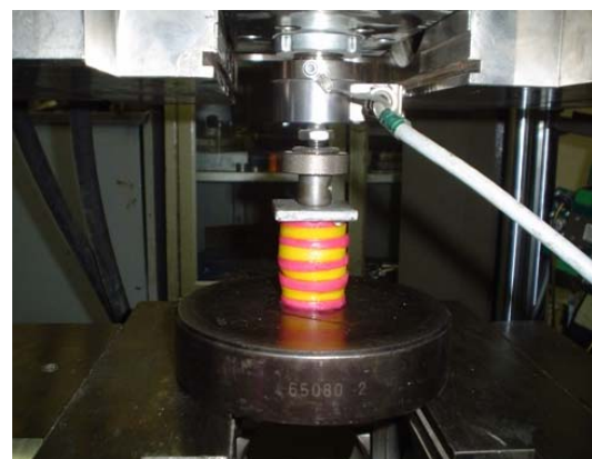
Fig. 3: Compression test performing on 60 ton press
