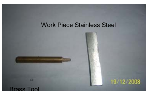
Fig 7. Work piece and tool before Machining
