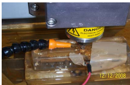
Fig 5. Electrochemical Machining Process going on.
