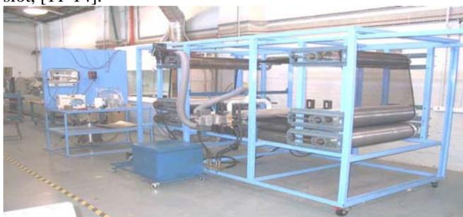
Fig 18: Photograph of microwave drying experimental set-up
